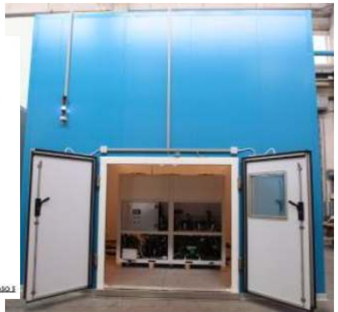
Figure 7: heat pump inside the testing room
