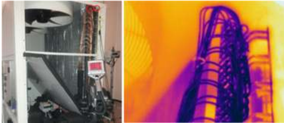
Figure 13. Coil position inside heat pump: (a) Thermocouple position, (b) Thermo-camera image
